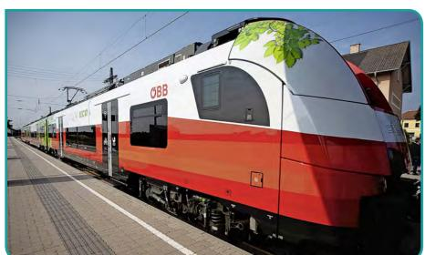
Siemens Mobility's Desiro ML OBB Cityjet eco electric-battery hybrid trains have been in passenger service with Austrian Federal Railways since August 2019.
