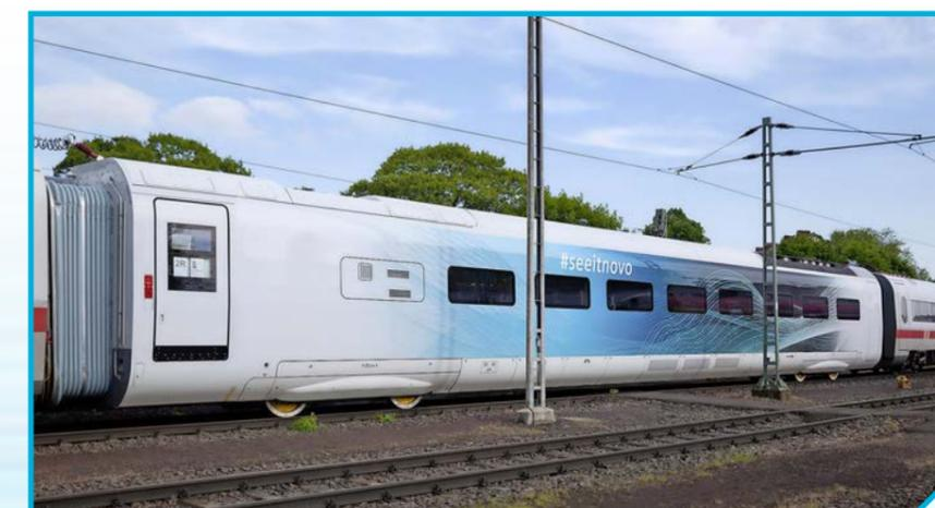
Siemens has been testing elements of the Velaro Novo design since April in its Novo test car that is currently incorporated into a DB-operated ICE S train on the German network. SIEMENS.
