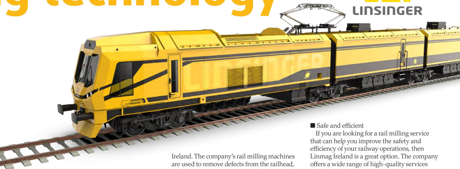
which occur due to train operation. Restoring the correct rail profile increases the smoothness of train operations, reduces undesirable forces and extends the rail life enormously. This reduces the Whole Life Cost and prolongs the intervals between expensive re-railing interventions.
