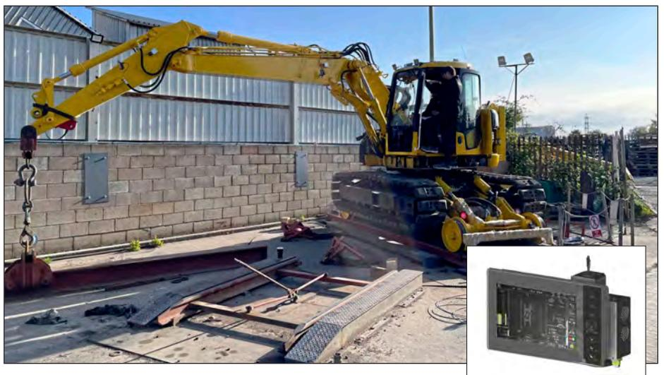
In addition to the RRCS, InTeEx also provides a pure Movement Limiting Device without RCI/RCL, called EC-S. This can be installed to almost all type of construction machinery, both on and off rail, in use of a Movement Limiting Device, for example excavators, wheel loaders, and MEWPs. If there is a need for a more basic and cost-efficient system without high safety features, the InTeEx EC-B would be a good alternative
