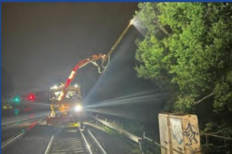
12m telescopic spray lance with large droplet oscillation and spray nozzles
