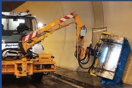
On-track plant, automated chemical delivery, less waste
